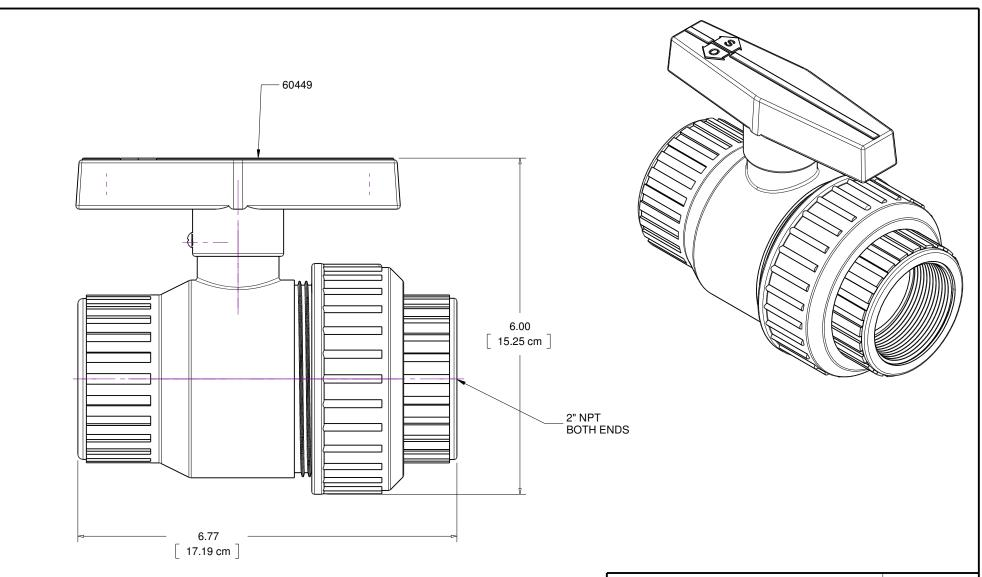
MATERIAL - POLYPROPYLENE WITH TEFLON SEATS EPDM O-RINGS
